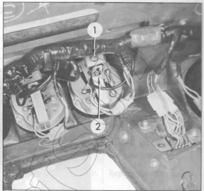
Fig. BE-19 Removing water temperature gauge and oil pressure gauge
