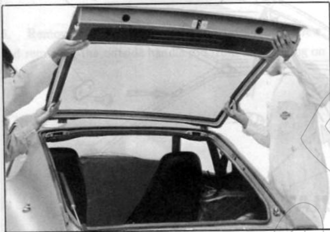
Fig. BF-38 Removing tail gate
