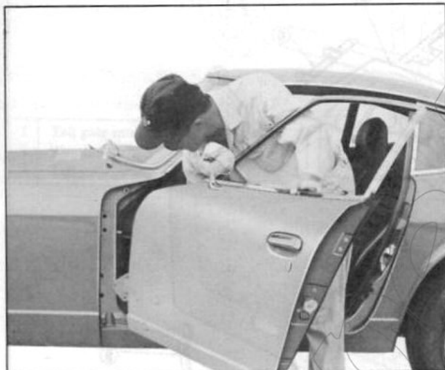
Fig. BF-19 Removing the door
