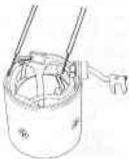
EE017 Fig. EE-17 Testing field coil for ground
