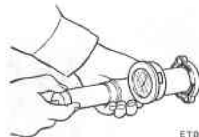
Fig. ET-12 Testing radiator cap
