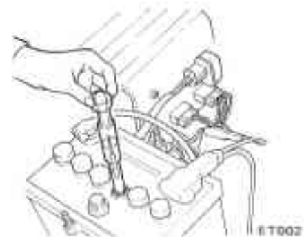
Fig. ET-2 Checking the specific gravity of battery electrolyte
