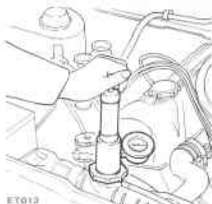
Fig. ET-13 Testing cooling system pressure
