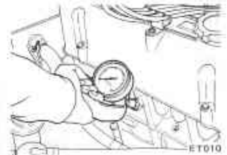
Fig. ET-10 Testing compression pressure
