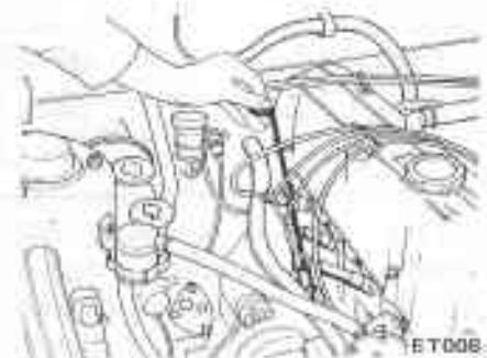
Fig. ET-8 Checking engine oil level
