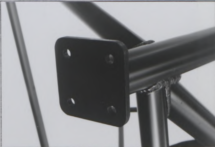
Rear support to bulkhead
