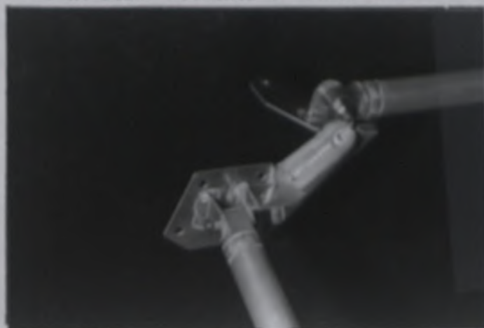
Front reinforcements to strut tower
