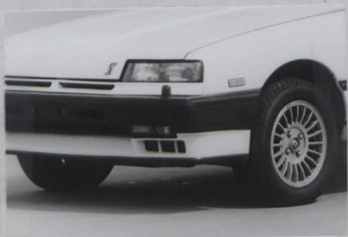
Photo: Air intake for cooling intercooler
