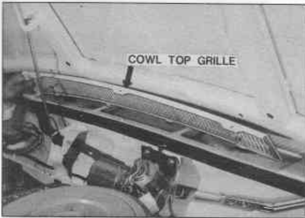
Fig. BE-33 Cowl top grille removal
