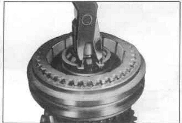
Fig. TM-19 Releasing 2nd and 3rd speed hub snap ring
