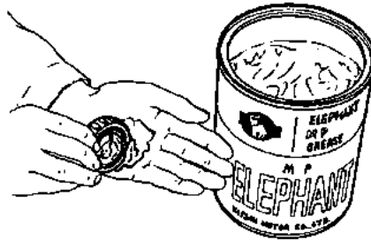
Fig. FA-10 Greasing bearing cone and roller assembly
