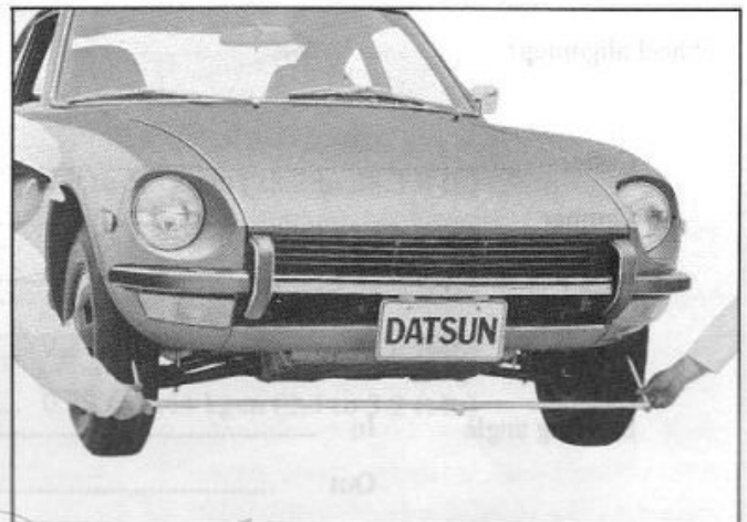
Fig. FA-50 Measuring toe-in
