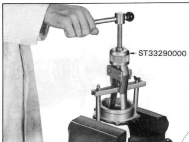
Fig. PD-6 Removing side bearing outer race
