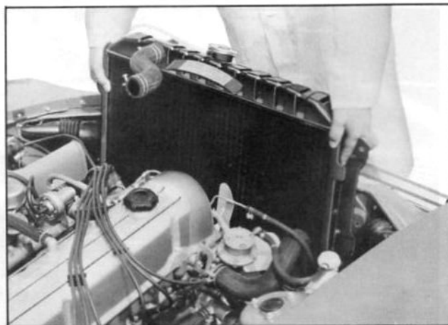
Fig. ER-2 Removing radiator
