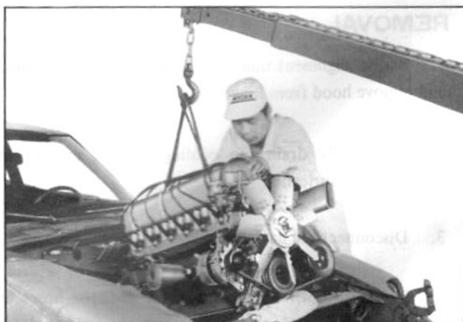
Fig. ER-6 Lifting engine
