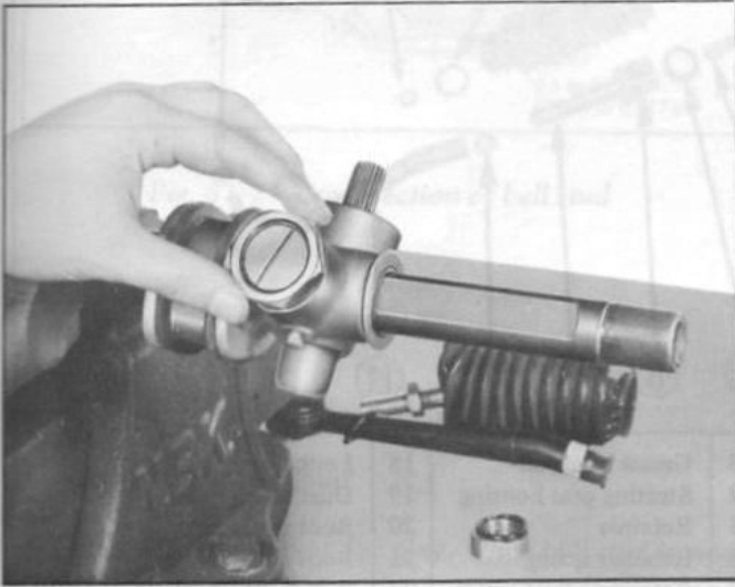
Fig. ST-18 Removing side rod outer socket
