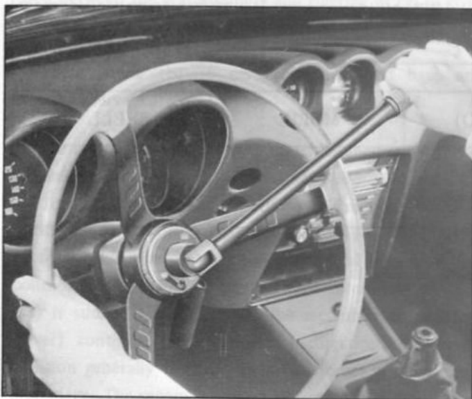
Fig. ST-3 Removing steering wheel
