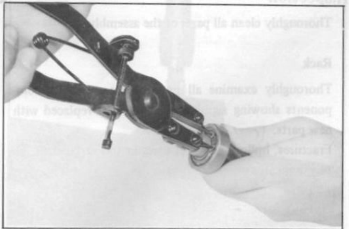
Fig. ST-22 Removing snap ring
