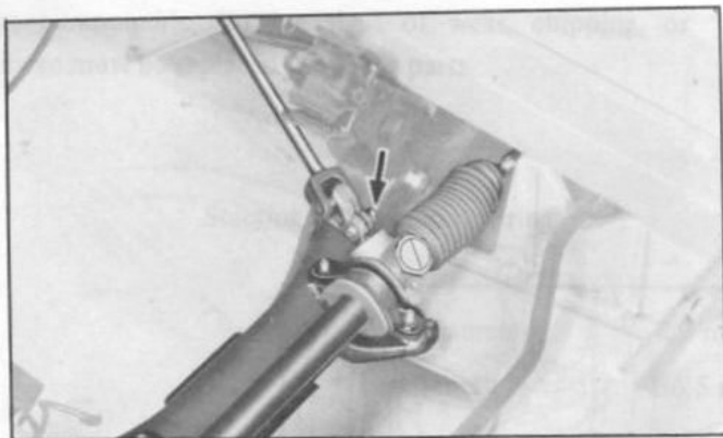
Fig. ST-13 Disconnecting lower joint from pinion
