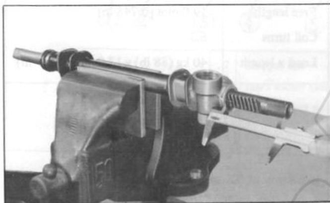
Fig. ST-26 Measuring protruding portion of rack
