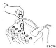
Fig. ET-5 Checking the specific gravity of battery electrolyte
