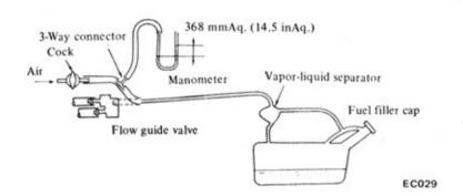
Fig. ET-14 Checking evaporative emission control system (for B210)
