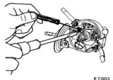
Fig. ET-6 Measuring point gap
