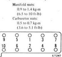
Fig. ET-1 Cylinder head bolt tightening sequence
