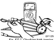
Fig. ET-7 Checking high tension cable
