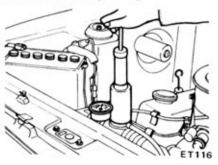
Fig. ET-13 Testing cooling system pressure
