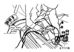
Fig. ET-8 Checking ignition timing
