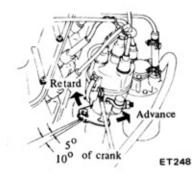
Fig. ET-9 Adjusting ignition timing
