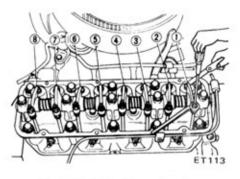
Fig. ET-3 Adjusting value clearance
