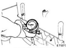
Fig. ET-2 Testing compression pressure
