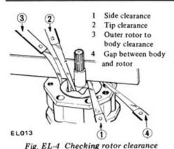
8. Place a straight edge across the face of pump as shown in Figure EL4. Check side clearance (outer to inner rotor) and gap between body and straight edge.
