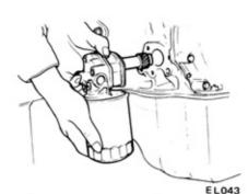
Fig. EL-2 Removing oil pump assembly
