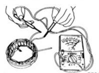
EE043 Fig. EE-31 Testing stator for continuity
