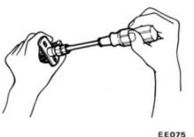
Fig. EE-60 Removing cam
