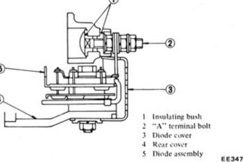
Fig. EE-38 Sectional view of diode and A terminal
