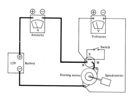
EE405 Fig. EE-17 Circuit of no-load test
