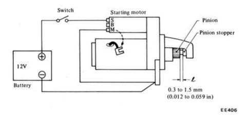
Fig. EE-18 Circuit of magnetic switch assembly test
