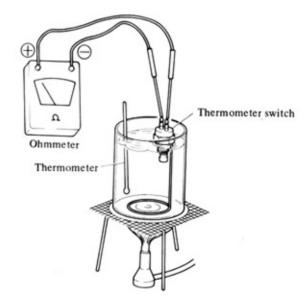
Fig. EE-63 Inspecting thermometer switch
