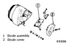
Fig. EE-27 Removing diode assembly
