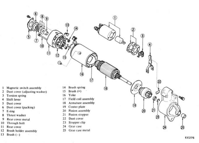
Fig. EE-6 Exploded view of starting motor
