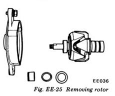
Pull rear bearing out from rotor assembly with a press or bearing puller.
