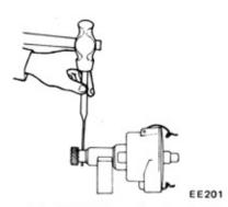
Fig. EE-58 Removing knock pin
