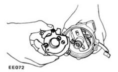
Fig. EE-57 Removing breaker plate
