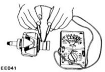
Fig. EE-29 Continuity test of rotor coil
