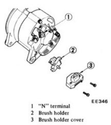
Fig. EE-23 Removing brush
