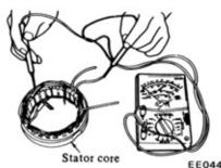
Fig. EE-32 Testing stator for ground
