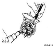
Fig. EE-52 Adjusting point gap
