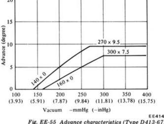
Fig. EE-55 Advance characteristics (Type D413-67)
