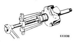
Fig. EE-26 Pulling out of rear bearing
