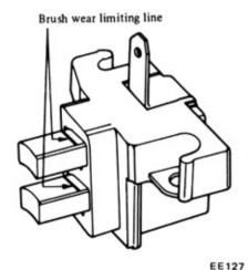
Fig. EE-36 Brush wear limit
