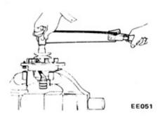
Fig. EE-39 Tightening pulley nut
