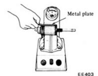
Fig. EE-14 Testing armature for short
