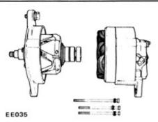
Fig. EE-24 Separating front cover with rotor from rear cover
