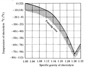
Fig. EE-5 Freezing point of electrolyte
