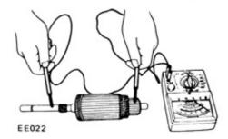
Fig. EE-13 Testing armature for ground
