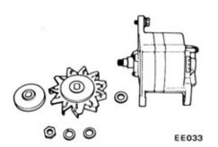
Fig. EE-22 Removing pulley and fan
