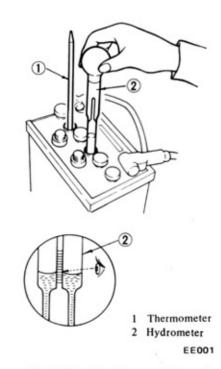
Fig. EE-2 Checking specific gravity
