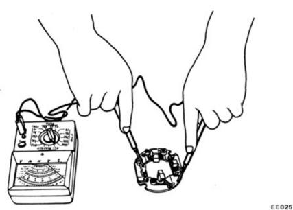
Fig. EE-16 Testing brush for ground
