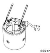
Fig. EE-10 Testing field coil for ground
