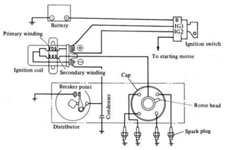
Fig. EE-48 Ignition system circuit
