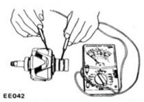
Fig. EE-30 Testing rotor coil for ground
