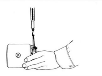
Fig. EE-11 Inspecting brush spring tension
