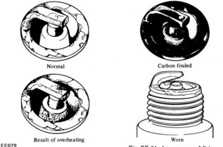
Fig. EE-61 Appearance of firing end
