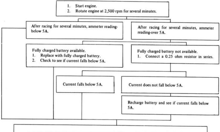
Reduce engine speed to idling and then raise it to 2,500 rpm while observing needle of voltmeter.
