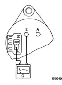
Fig. EE-28 Inspecting alternator
