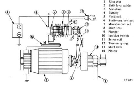
Fig. EE-1 Starting circuit
