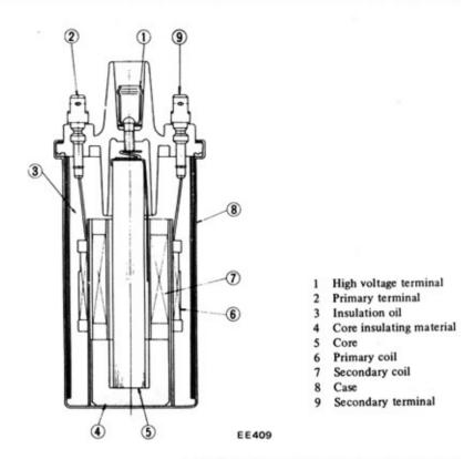
Fig. EE-49 Cross-sectional view of ignition coil
