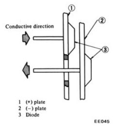
Fig. EE-33 Conductive direction of diode
