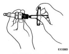
Fig. EE-62 Measuring spark plug gap
