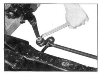
and release the nut at each end of the rod and then slightly tap the rods clear of the levers to which they are connected.
