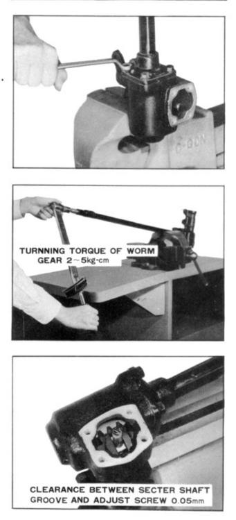
Fitting the side cover with adjust screw, fix the side cover to gear box by turning it for left way.
