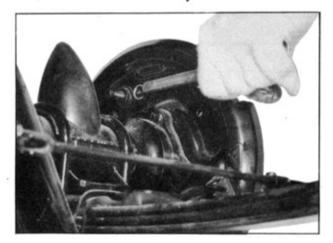
To remove the wheel cylinder, detach the spring at side brake cross rod and pull out the pin of cross rod end.
