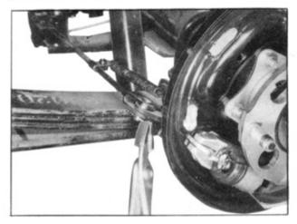
Disconnect the brake tube from back of flange.
