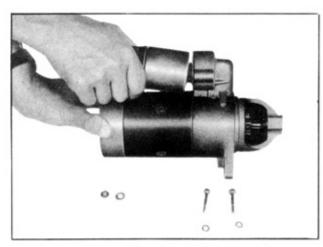
Removing Magnetic Switch
