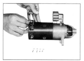
Drawing out Brushes (After removing fixing screw)
