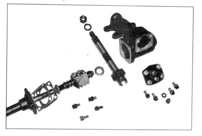
Components of Sceering Gear Housing
