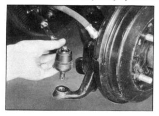
Rotating the gear arm several times for right and left way to find and correct center without any variation about back-lash.
