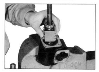
Insert the ball nut assembly with the worm bearing at rear side into the gear housing and smear the oil to the worm bearing.
