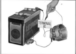
Check between the lead wire and the diode set common with the other 2 diodes or the rear cover with the lamp and battery. It is all right if one side flares and the other is off. If both sides flare, there is short circuit and both sides are off, there is open.
