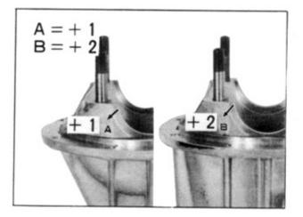
Measure the back lash of the drive pinion & ring gear as Figure by using the dial indicator to make sure that if is within 0.1 mm-0.2 mm (0.004''-0.008''). If it is much, move to left by taking off the right shim, for adjustment.
