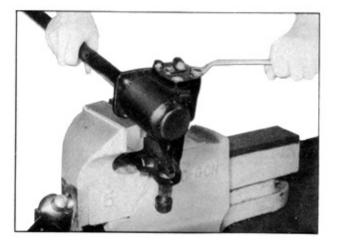
Unscrew the lock nut of adjusting screw, and then take off the side cover.
