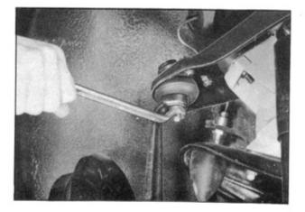
Remove screen of the hood ledge and then unscrew the bolt of upper link spindle.
