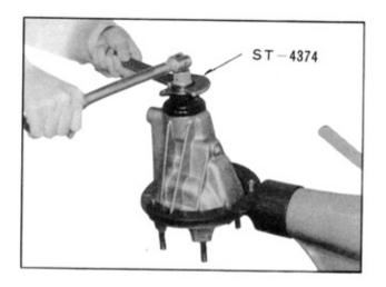
(2) Mount the front bearing outer race in the carrier.
