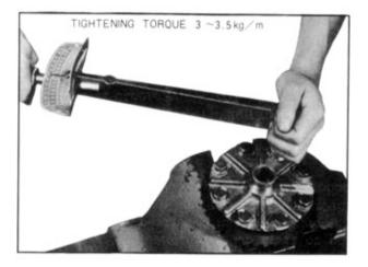
Mount the side bearing in the differential case.
