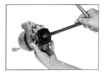
d) Remove the hex. nut of pulley and pull off the pulley and the half-moon key. Be careful not to injure the fan when the nut is removed. e) Remove the through bolt tightening bolt front cover and rear cover, pull off the front cover and rotor.
