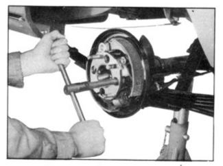
Remove of Axle Shatt and Disc Assembly
