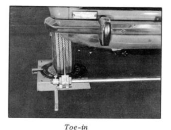
Toe-in  $2 \sim 3 \text{ mm}$ Camber 1°45' Caster 2°15' King pin angle 6°30' Side slip Less than 3 mm with each running distance 1 mm Turning angle (Inside) 45° (Outside) 36°36' Rotation torque front Less than 9 kg-cm hub (Motive) Clearance of front hub to direction along Less than 0.08 mm the shaft Clearance of ball joint to direction along Less than 0.9 mm the shaft
