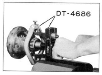
Using of Side Bearing Puller (DT-4686)
