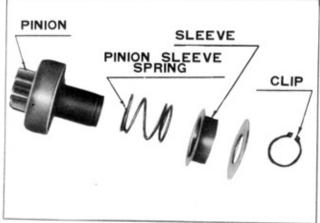
Disassembling Pinion Subassembly
