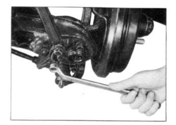
Screw out the attached nut at a front side of tension rod (Leave alone other side nut).
