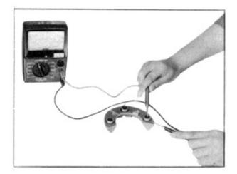
Check resistance with the tester between the diode base commonly used for 2 diodes and lead wire on the rear cover -2 times charging the poles
