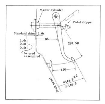
pedal should be adjusted by the adjusting shims.
