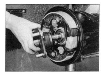
Pack the hub with recommended grease. Replace the hub oil seal over the inner bearing. Renew the seal if it is damaged.
