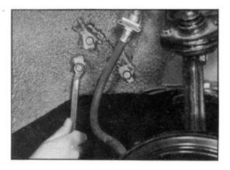
After the side and cross rods disconnected the idler can be detached from the body.
