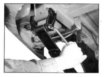
Connect the rear side of spring to the bracket.
