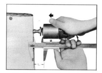
Measurement of Plunger Gap
