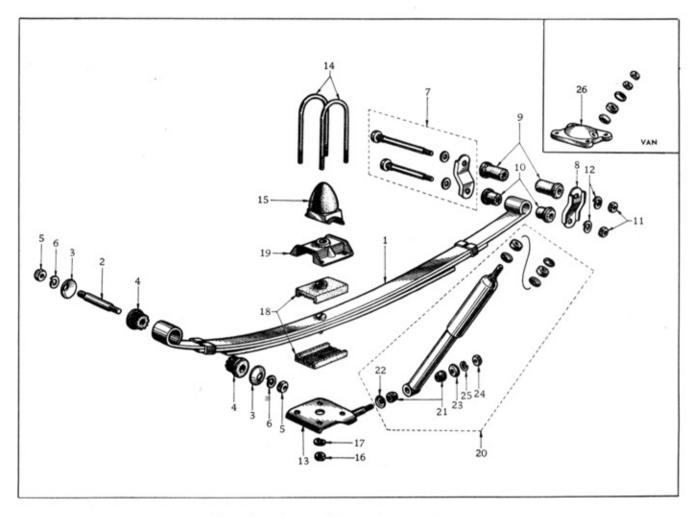
Constructure of Rear Suspension
