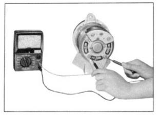
Check between the terminals, A-N as shown in Figure. Set the dial of tester for conductivity and put the tester needles at both terminals alternately.
