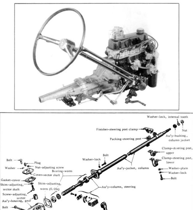
Components of Steering Gear Box
