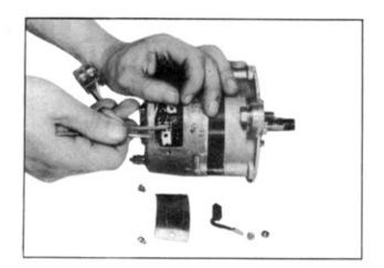
c) Remove the cover of bearing and take off the hex. bolt of shaft.
