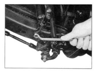
Screw out the bolts (2) at the side of lower link on the tension rod.
