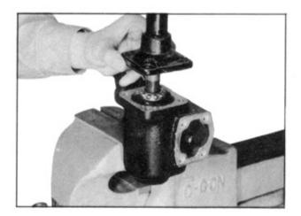
Select the same thickness of shims at the disassembling time and connect the column assembly with it to the gear housing.
