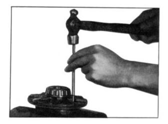
2) Fix the drive gear (Ring gear) with the differential case.
