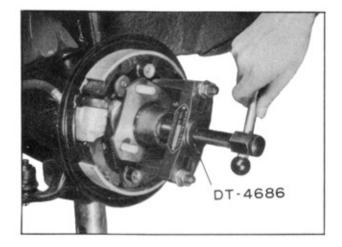
After the hub removed, the bearings can be dismantled. The inner bearing and oil seal can then be removed by inserting the drift from the opposite side of the hub.
