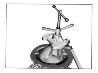
Tool No. DT4782, DT4631 & DT4689 Pull out the Bearing Race
