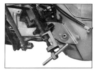
The gear arm must not be hammered from its shaft.
