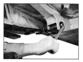
Attach the bushing to the rear spring and rear spring bracket.
