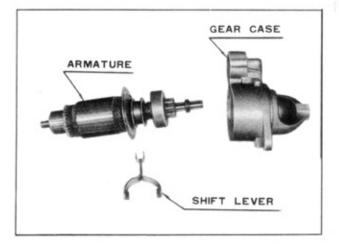
Disassembling Armature and Gear Case
