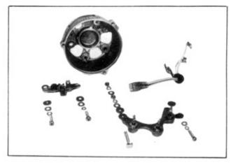
Remove the diode set and brush holder from the rear cover.
