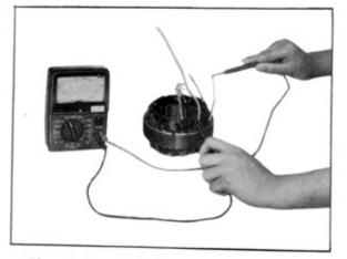
If each terminal of the coil and the terminal connected to N terminal are not conductive, that is all right.
