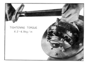
So far, only the differential unit is mounted and the drive gear is locked with the drive pinion, therefore, the following adjustment must be made to acquire the regular side bearing preload & the gear back lash.
