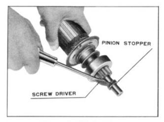
Removing Pinion Stopper
