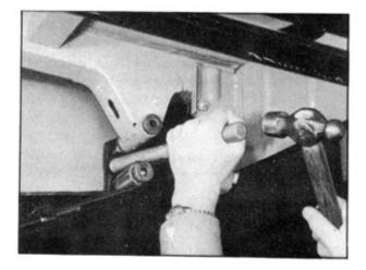
Disconnect the shackle, rear spring front pin and then separate the rear spring as showing the figure.
