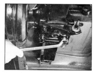
Take off the shock absorber from spring seat. Jack up the rear axle housing to release load. Disconnect bumper, U bolt, location plate, seat pad and spring seat etc.
