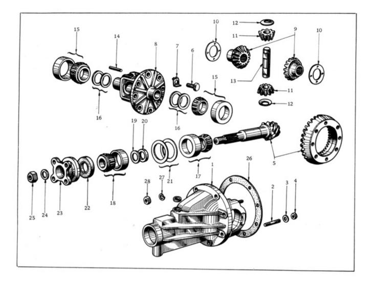
Gear Carrier & Gear
