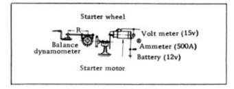
Torque Testing Apparatus
