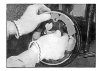
Detach the return spring and remove brake shoes.
