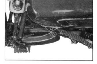
Supporting the front spring, remove the lower link pin at the unscrewed side of tension rod.
