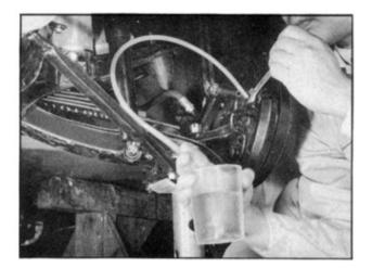
Push out the bleeder valve several turns and work on the brake pedal, depressing it quickly and releasing slowly repeatedly until no air bubbles are evacuated from the bleeder valve.
