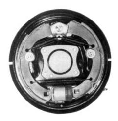
The hand brake is of mechanical two rear wheel braking type and is equipped with a stick-shaped handle for R.H. Drive and a floor lever type for L.H. Drive.
