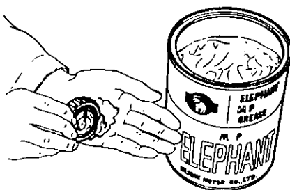
Fig. FA-10 Greasing bearing cone and roller assembly
