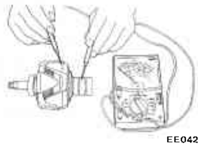
Fig. EE-42 Testing rotor coil for ground
