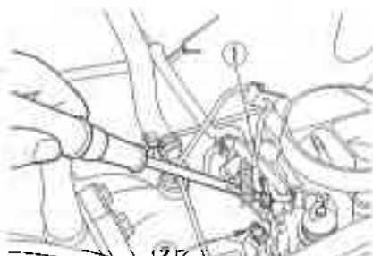
1 Throttle adjust screw 2 Idle adjust screw EF015 Fig. EF-15 Idling adjustment
