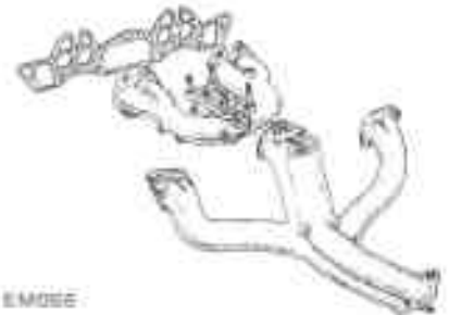
Fig. EM-11 Manifolds for single carburetor
