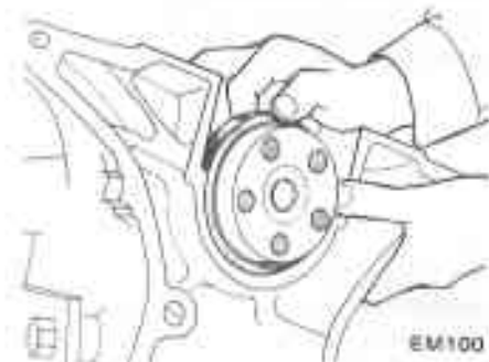
Fig. EM-25 Removing rear oil seal
