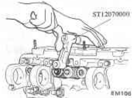
Fig. EM-31 Removing valve
