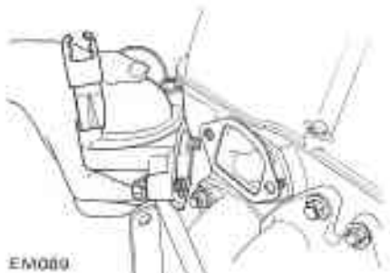
Fig. EM-14 Removing thermostat housing
