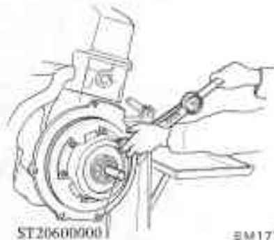
Fig. EM-107 Installing clutch assembly
