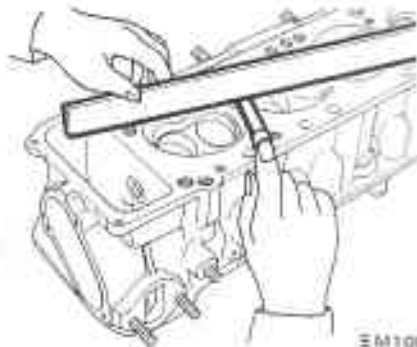
Fig. EM-34 Checking cylinder head surface
