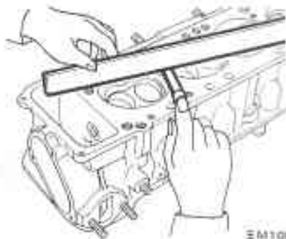
Fig. EM-34 Checking cylinder head surface
