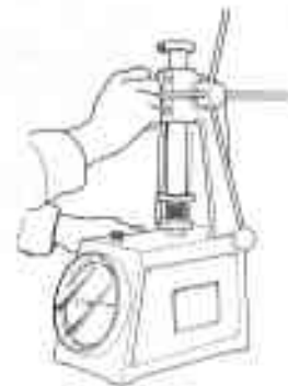
Fig. EM-39 Measuring spring tension
