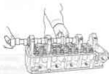
Fig. EM-30 Removing camshaft
