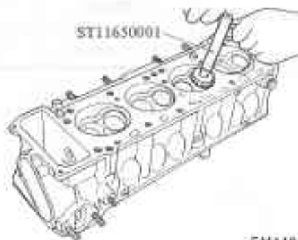
EM118 Fig. EM-44 Correcting valve seat
