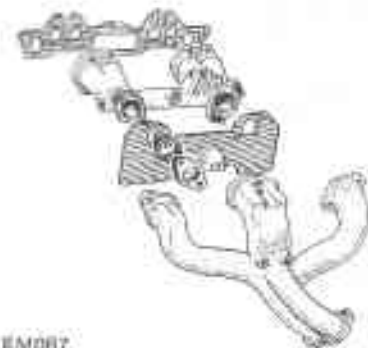
Fig. EM-12 Manifolds for twin carburetor
