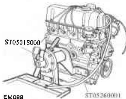
Fig. EM-13 Engine on engine stand
