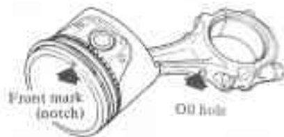
Fig. EM-85 Assembling piston and connecting rod
