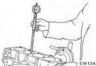
Fig. EM-51 Measuring cylinder bore diameter
