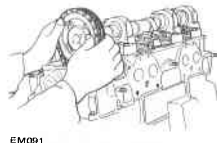
Fig. EM-16 Removing camshaft sprocket
