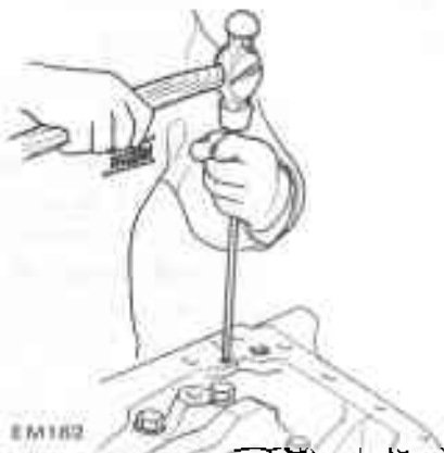
Fig. EM-90 Driving side oil seal
