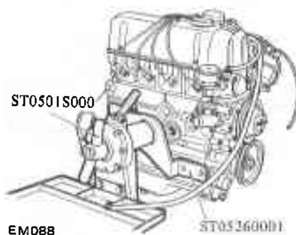
Fig. EM-13 Engine on engine stand
