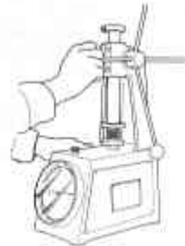
Fig. EM-39 Measuring spring tension
