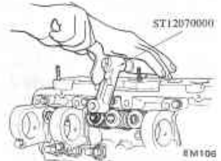
Fig. EM-31 Removing valve
