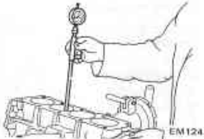
Fig. EM-51 Measuring cylinder bore diameter
