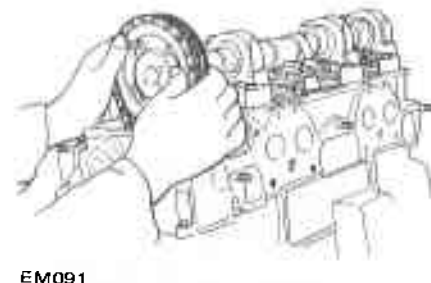
Fig. EM-16 Removing camshaft sprocket
