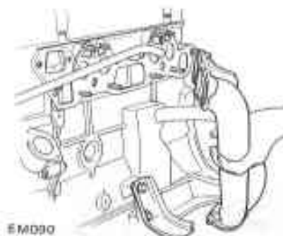
Fig. EM-15 Removing manifolds
