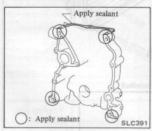
e. Before installing front cover, align locating notches.
