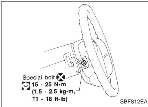
7. Position air bag module and tighten with new special bolts.
