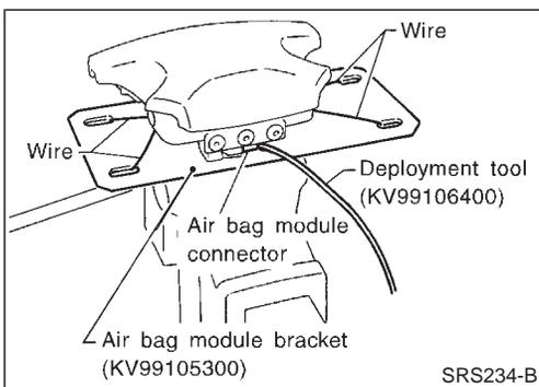
3. Connect deployment tool (SST: KV99106400) to air bag module connector.
