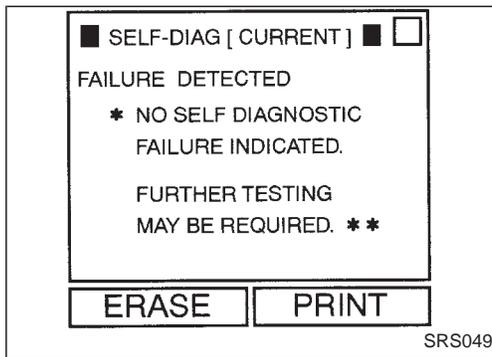
If no self-diagnostic failure is detected on “SELF-DIAG [CURRENT]” even though malfunction is detected in DIAGNOSTIC PROCEDURE 1, check the battery voltage. If the battery voltage is less than 9V, charge the battery. Then go to DIAGNOSTIC PROCEDURE 3, page RS-31. If the battery voltage is OK, go to DIAGNOSTIC PROCEDURE 4, page RS-33, to diagnose the following situations:
