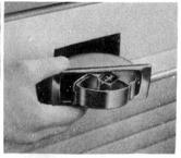
Ash trays, installed in the center of the dashboard and in both sides of the rear seat, can be removed for cleaning.
