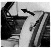
Tilt the front seat by lifting up the safety lock lever.
