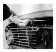
Pull the hood lock handle located at the lower right-hand side of the instrument panel, and then the safety catch, located under the center edge of the hood, must be pushed up to completely release the hood.
