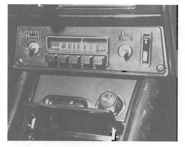
Figure V-2. Radio Tuner Mounting Screws
