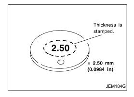
New adjusting shims have the thickness stamped on the rear side.
