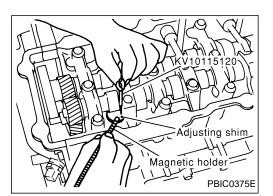
8. Remove the adjusting shim by using a magnetic holder.
