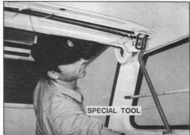
Fig. BF-20 Removing torsion bar
