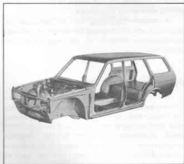
Fig. BF-2 510 Series body structure (wagon)
