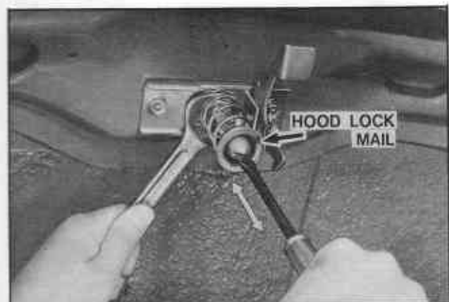
Fig. BF-9 Adjusting male plunger
