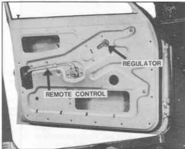
Fig. BF-13 Front door showing remote control link
