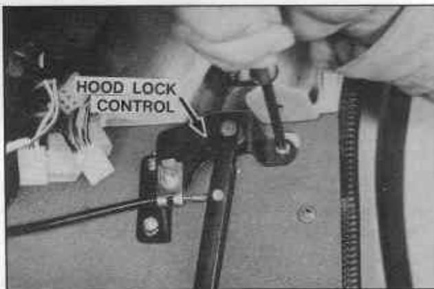
Fig. BF-8 Removing the hood lock control
