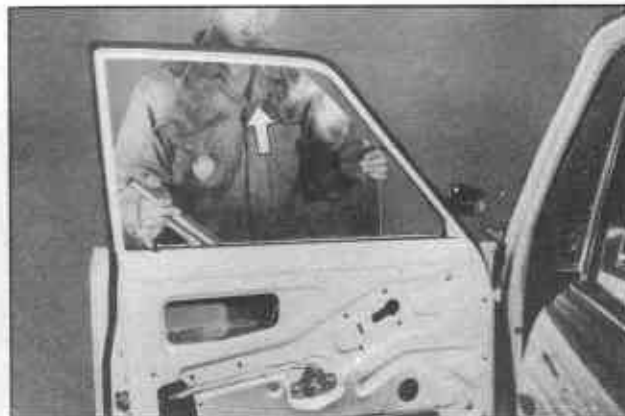
Fig. BF-15 Removing window glass
