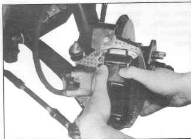
Fig. BR-20 Removing anti-rattle clip
