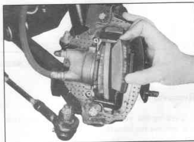
Fig. BR-22 Removing pad
