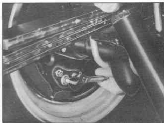
Fig. BR-36-b Adjusting rear brake - station wagon
