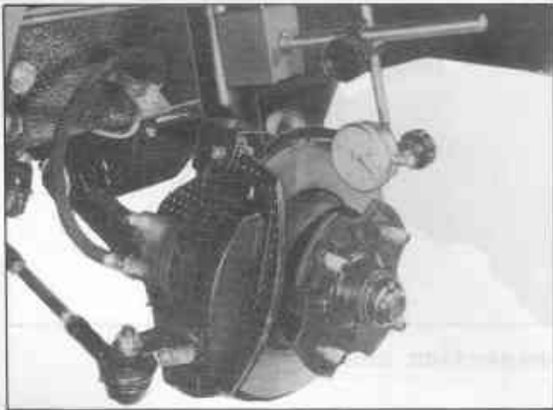
Fig. BR-18 Measuring run out of disc
