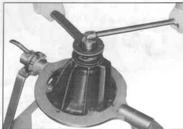
Fig. PD-42 Removing drive pinion unit
