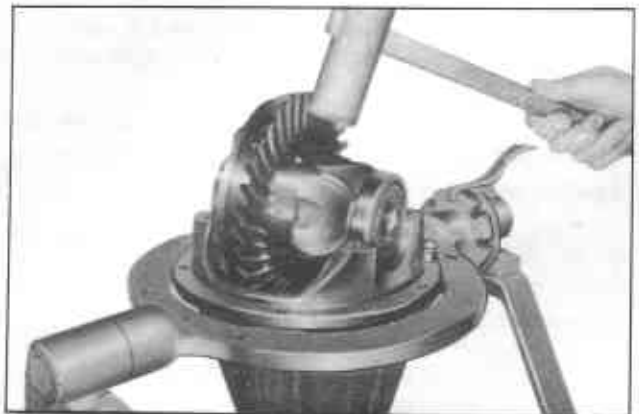
Fig. PD-47 Installing differential case assembly
