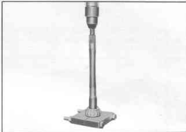
Fig. PD-12 Removing rear bearing inner race
