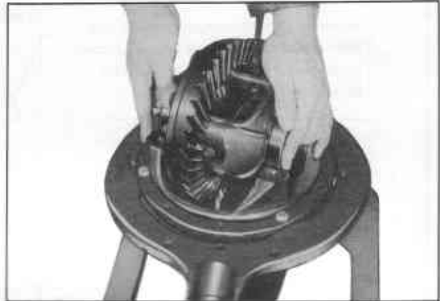
Fig. PD-37 Removing differential case assembly
