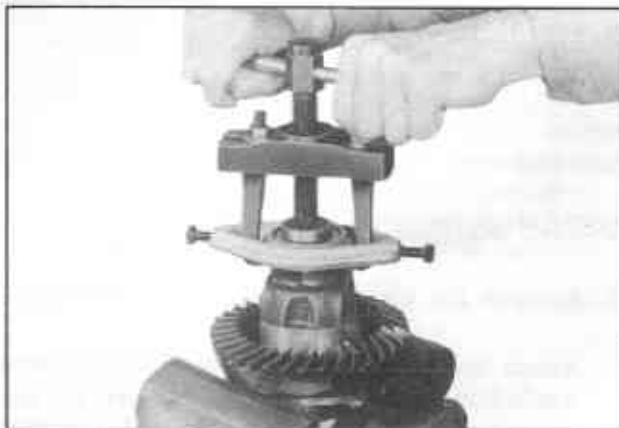
Fig. PD-13 Removing side bearing cone
