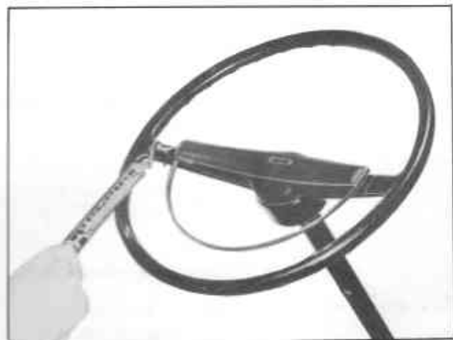
Fig. ST-12 Measuring initial turning torque
