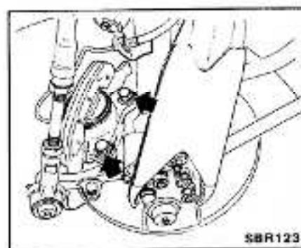
2. Remove yoke holder, retaining rings and dust seals from both pistons.
