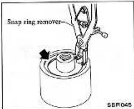
7. Disassemble inner piston by removing snap rings A and C.
