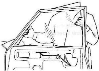
Fig. BF-35 Removing door window glass
