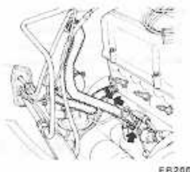
Fig. ER-2 Air conditioner water hoses
