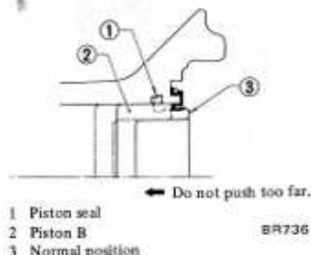
Fig. BR-2 Position of piston
