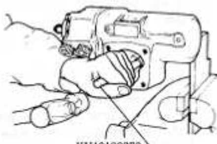
Fig. ST-17 Installing oil seal
