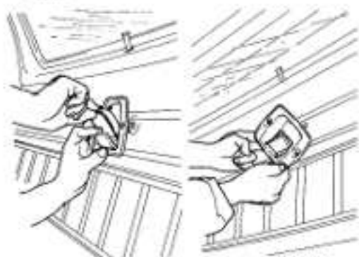
Fig. BE-24 Removing tail gate trim
