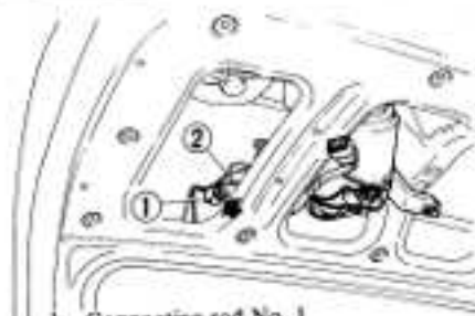
Fig. BE-25 Disconnecting wiper motor unit
