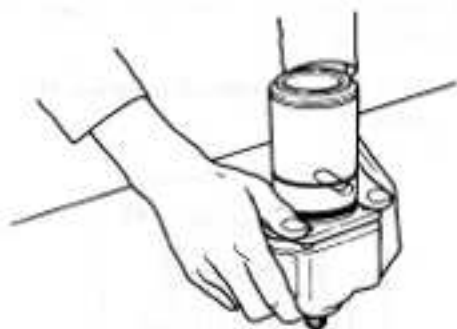
Fig. ST-24 Removing rear housing
