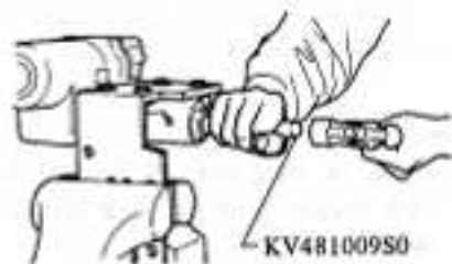
Fig. ST-16 Installing oil seal
