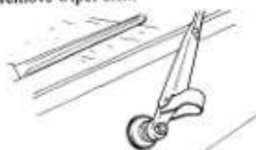
Fig. BE-23 Removing wiper blade
