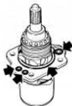
Fig. ST-27 Installing O-rings
