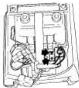
Fig. BE-12 Removing console box lamp switch
